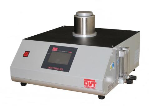
USED TO EXAMINE STRUCTURAL DETERIORATION IN PLASTICS DUE TO THERMAL AND OXYGEN EFFECTS
